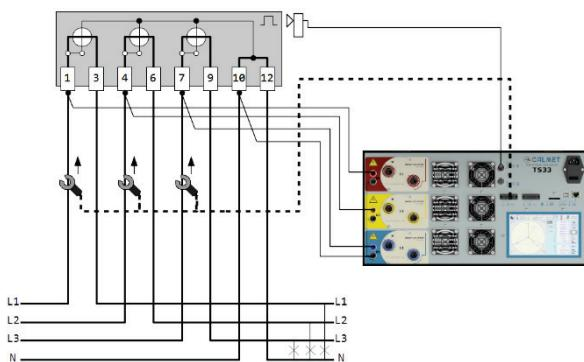
The use of TS33 as a stand-alone reference meter for Current Transformer testing
