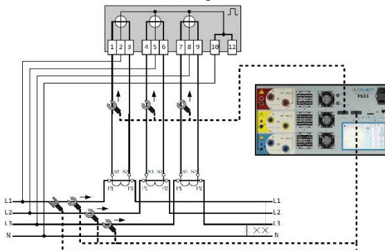
The use of TS33 as a reference meter together with the integrated power source for electricity meter testing
