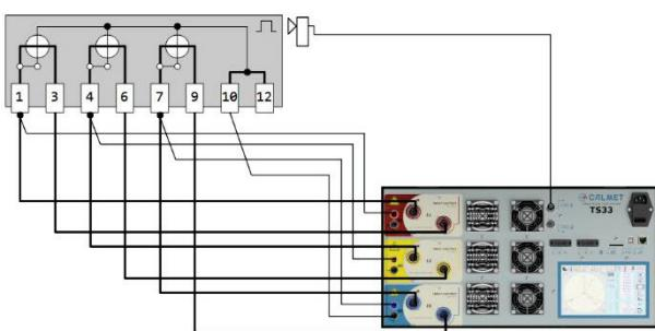
The use of TS33 as a voltage meter and three phase current source for electricity meter testing
