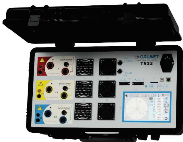
The Calmet TS33 portable test system consists of a three-phase reference meter of accuracy class 0.04% (or 0.1%) and an integrated three-phase current and voltage source up to 3x120A/600V. The TS33 is designed for analysis of complete metering installations and local mains conditions.
